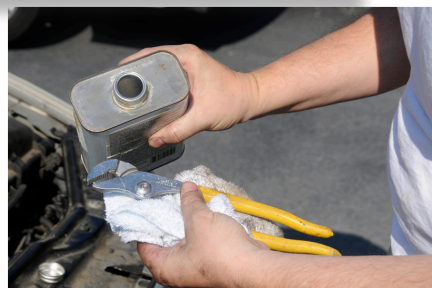
Oily surfaces can be cleaned if a solvent is used that is completely miscible with the oil.
