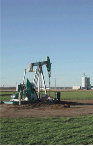
NETL is demonstrating carbon dioxide flooding EOR in the Hall-Gurney field in Russell, Kansas, using carbon dioxide recovered from a nearby ethanol plant.
